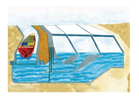
Where do you think the water that fills the tank comes from? It comes from where the Cheetah is, right now. Normally, water is stored in a large cistern next to the canal, and every time a ship moves to each level, the water flows out and fills the tank. There are a total of 18 large water storage areas - nine for each gate.
