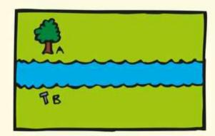
Drive a stake (B) into the ground on your side of the river in line with the tree.
